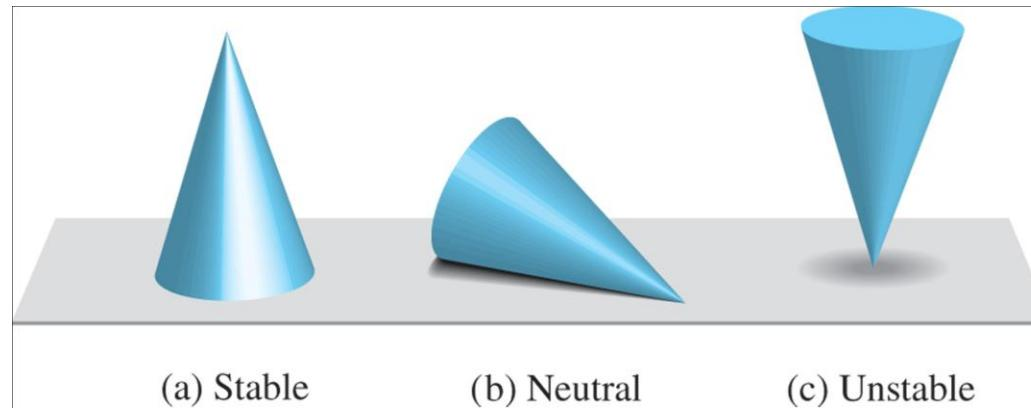
Response to a displacement/initial condition will produce either a decreasing, neural, or increasing response.
