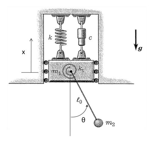
Two independent coordinates :  $q_1 = x, q_2 = \theta$  (2 *pts*)  $Q_1 = 0$  and  $Q_2 = 0$  (2 *pts*)  $R_x = \frac{1}{2}c\dot{x}^2$  and  $R_\theta = 0$  (4 *pts*)
