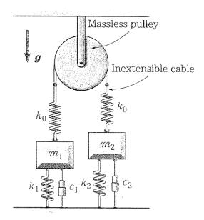
A possible definition of the coordinate system is shown below, with  $x_p$  defined as the displacement of the pulley, and  $m_p$ , the mass of the pulley, equals to zero.
