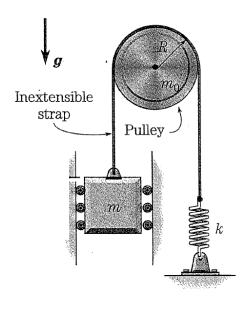
There are two masses and one spring, however, because the disk moves without slipping, the distance that it rotates is equal to  $r\theta$ , which is equal to the distance x traveled by the mass m. Thus, m and m<sub>0</sub> can be combined. Together with the spring, the system has two energy storage elements, and is a second order system.
