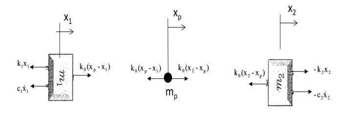
Assuming that gravitational force is much less than inertial, spring, and damping forces, and using Newton's Second Law gives:
