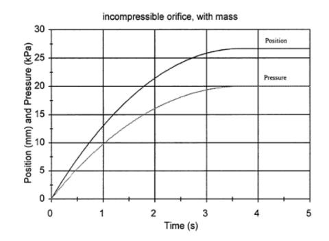
Model of system using compressible orifice equation (incompressible approximation) with mass:
