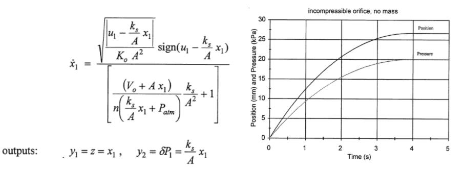
Model of system using incompressible orifice equation with mass:
