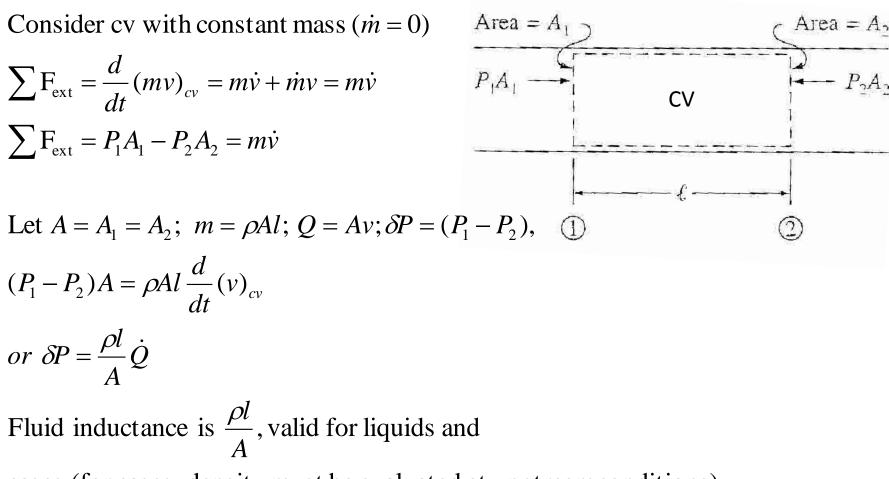
gases (for gases, density must be evaluated at upstreamconditions)
