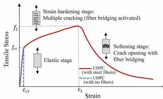
Fig. 2. UHPC stress-strain diagram (Kaka et al., 2016)
