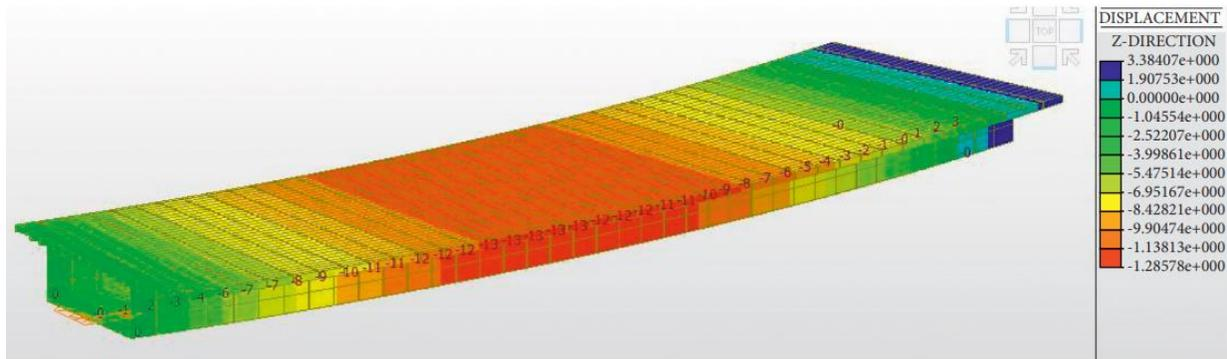
Fig. 3. Example finite element model of concrete bridge girders (Wang et al., 2022)
