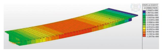
Fig. 3. Example finite element model of concrete bridge girders (Wang et al., 2022)
