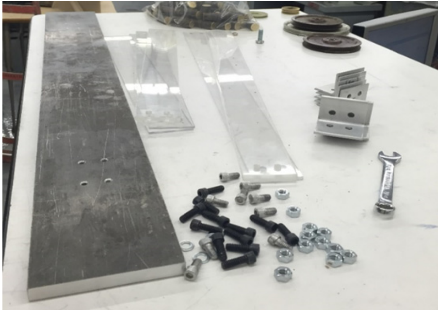
Fig. 2 Materials used in the construction of the single-story, single-bay portal frame.
