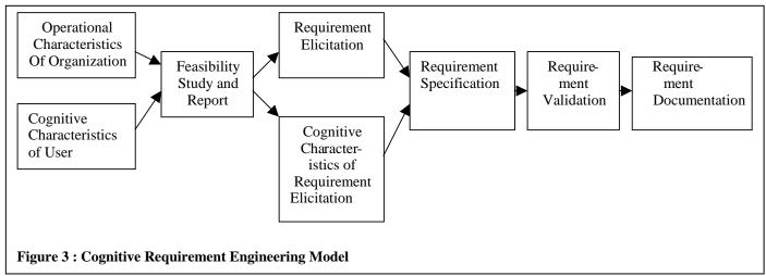
The requirement-engineering model is depicted in fig. 3. The person who is the catalyst behind the request for the software will play a key role in extending the need analysis and hence carrying out the requirement analysis. Once proper requirement engineering has been carried out, we can safely proceed to problem analysis. This will reduce the amount of rework.
