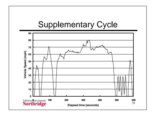
This cycle has nothing to do with fuel economy. It was added to the emissions test procedure starting with the 2002 model year. This cycle will test vehicles in high power operation to ensure that they meet the emission standards in real-world driving. The certification emissions from the federal test procedure (FTP), shown on the previous slide, are computed in the following manner:
