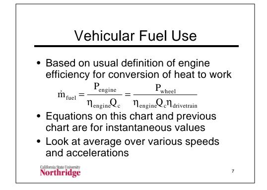
The equations for vehicle power on the previous slide and the equation above for the fuel use guide us seeking ways to reduce fuel use. Simply reduce all the items that are in the numerator and increase all the items that are in the denominator.
