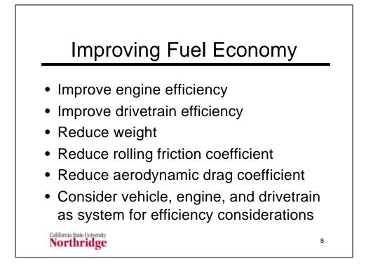
All of the ideas listed above follow from a simple consideration of the equations that are used to determine fuel consumption. However we have to examine the relationship among the engine, the drivetrain, and the vehicle to really see how the various components of fuel economy reduction interact.
