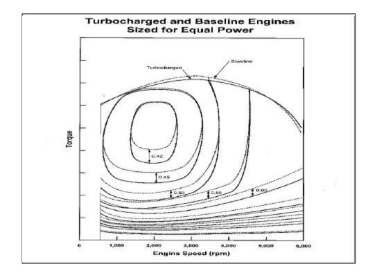
This chart shows the effect of adding a turbocharger to an engine that has been redesigned to produce the same power as an engine without a turbocharger. In this case the engine has higher efficiency when operating at low load points.
