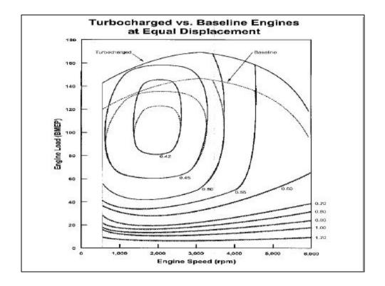
This chart shows the effect of adding a turbocharger to an engine. It is able to process more air and this produce more power than a naturally aspirated engine. This chart is based on the assumption that a turbocharger is added to the engine and no other changes are made in the size of the engine. This would increase the peak power of the vehicle, but would not make any significant change in the fuel economy.
