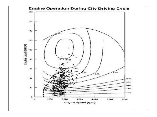
This chart shows the second-by-second operating points on the EPA urban driving cycle that is used for measuring fuel economy. The chart was generated using the actual speed versus time trace to define the load on a vehicle. (This cycle is shown later in this presentation.)
