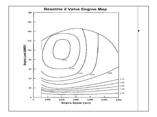
This is a typical plot of engine efficiency (or rather the inverse of efficiency as measured by the bsfc), known as an engine map. This one is for a typical mid-size vehicle such as a Ford Tarus. The actual data for the engine map is taken from composite data from various manufacturers that were averaged to maintain confidentiality.
