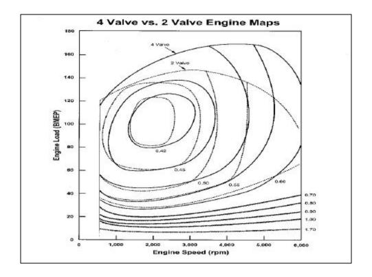
This chart is similar to the next to last chart. That chart showed the effect of adding a turbocharger to an engine without changing its size. It is able to process more air and this produce more power than a naturally aspirated engine. Here we assume that we add two additional valves to the engine without changing its displacement. The added valving allows the engine to process more air. This increases the peak power of the engine, but does not improve the fuel economy.
