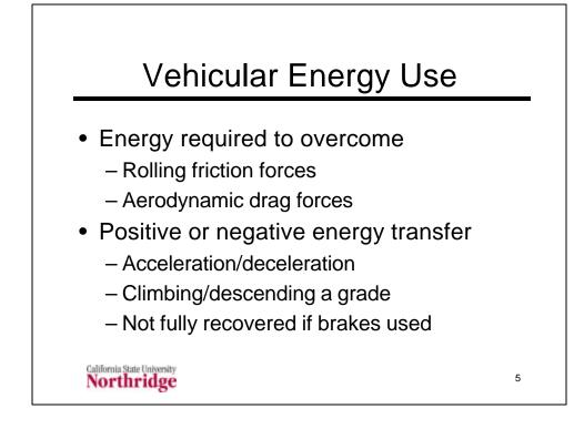
Energy is provided to the drive wheels of a vehicle to overcome resistances due to rolling friction and aerodynamic drag. The energy used to overcome these forces is transformed into heat and cannot be recovered.
