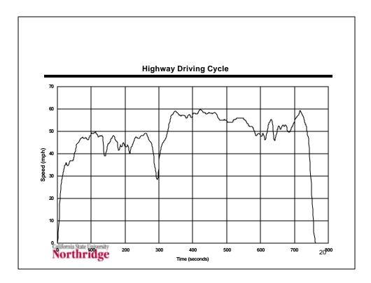
This is the cycle used for the highway fuel economy test. You can see that it has very little high speed driving that is encountered on a typical modern freeway outside an urban area (or inside an urban area outside of rush hours.) The discrepancy between the operation over this cycle and actual highway driving leads to an adjustment in the reported fuel economy that is only 78% of the fuel economy measured on this cycle.
