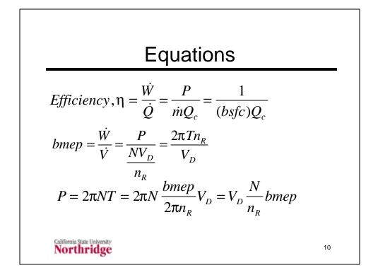
In these equations we have introduced two new variables. The first,  $V_D$ , is the displacement volume, the volume swept by the piston. This is the volume that we would plot on a thermodynamic P-v diagram.
