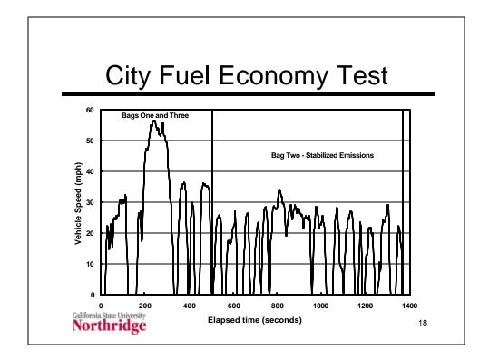
This chart shows the driving cycle that is used for the city fuel economy test. It was originally developed for testing cars and light duty trucks for emissions in a typical urban environment.
