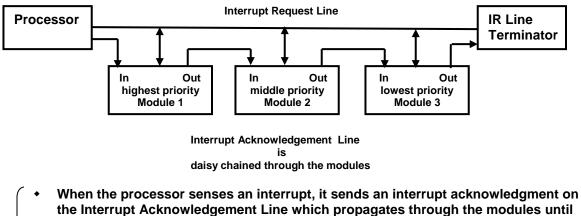
the Interrupt Acknowledgement Line which propagates through the modules until it reaches the requesting module, i.e., the module that sent the interrupt
